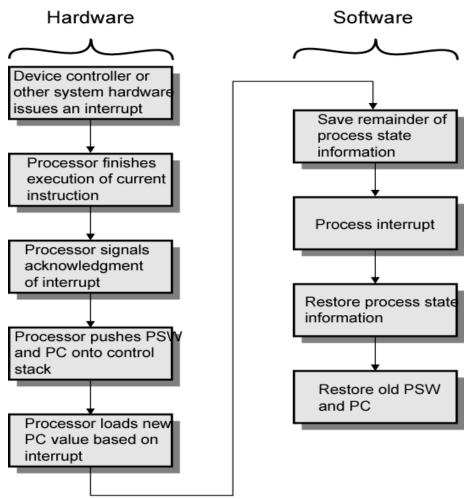
Fig: Simple Interrupt Processing
