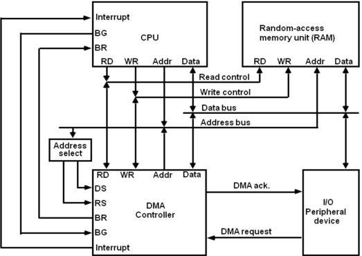
Fig: DMA transfer in a computer system
