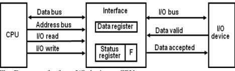
Fig: Data transfer from I/O device to CPU
