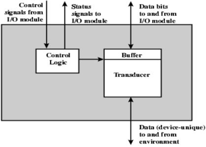
Fig: Block diagram of Peripheral device
