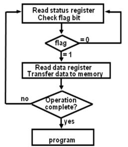
Fig: Flowchart for CPU program to input data
