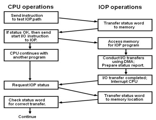
Fig: CPU – IOP communication
