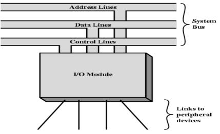
Fig: Model of I/O module
