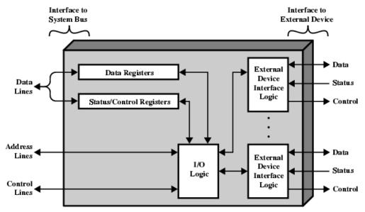
Fig: Block diagram of I/O Module
