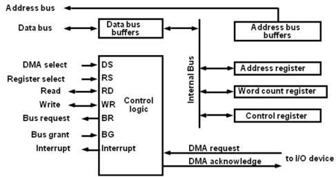
Fig: Block diagram of DMA controller
