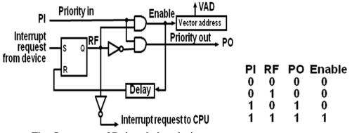
Fig: One stage of Daisy chain priority arrangement
