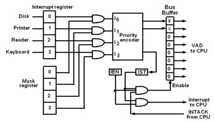
Fig: Parallel priority interrupts hardware
